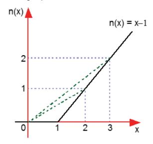
Therefore, one way of approximating the nonlinear model would be to consider the linear transfer function, for a model, where the gain of the feedback circuit was changed. Increasing the amplitude of the input in a nonlinear model would be equivalent to an increased gain, and vice versa for a decrease in the amplitude. We will use the method in the analysis, below.
