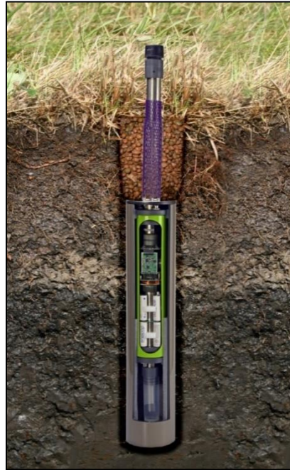
S3 Fig B. EDAPHOLOG probe with clay granule bag as matrix between the soil and the trapping system. The trapping tube is made by a purple net to prevent clay granules falling into the trap.
