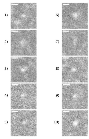
Particle diameters of the oligomers were measured as Feret's statistical diameter [1], using the software ImageJ 1.50d (NIH, USA, https://imagej.nih.gov/ij/). The average diameter of the oligomers is  $9.9 \pm 1.5$  nm, based on analysis of the 10 particles shown above. The scale bars in the images denote 10 nm.
