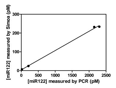
S7 Figure. Correlation of concentration of synthetic calibrator for miR-122 spiked into serum determined using Simoa and PCR ( $r^2 = 0.998$ ).
