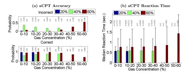
Figure 6. Relationship Between N<sub>2</sub>O Gas Concentration and Responsiveness. (A) Dependence of aCPT accuracy on reaction time. (B) Dependence of median aCPT reaction time on gas concentration. In (A) the top and bottom y-axes represent the probability of 'incorrect' and 'correct', respectively, for a given gas concentration bin. (B) error bars indicate  $\pm$  one standard deviation. The legend indicates different peak gas concentration groups.
