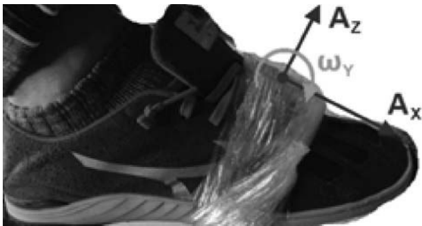
Figure 1. A shoe with the sensor, wrapped in food wrap film, attached to it. The arrows represent the directions in which the signals are measured. The missing arrows ( \omega_x , \omega_z and A_y ) can be derived using the right-hand rule for axis orientation.
