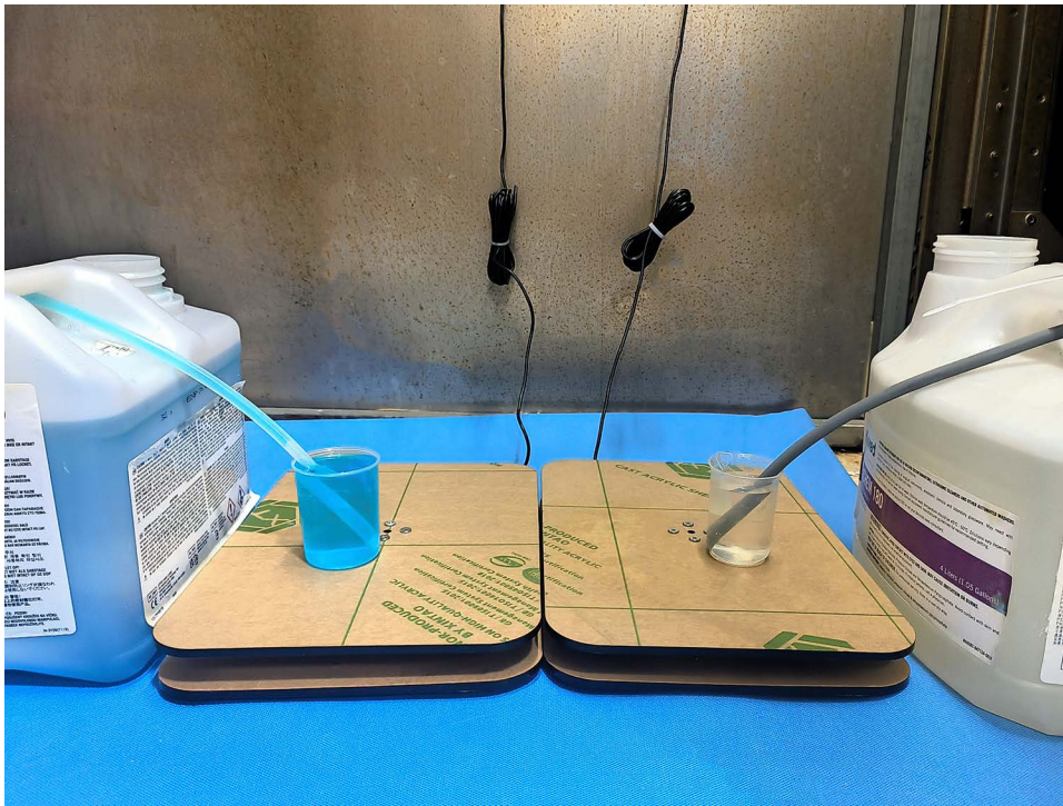
Fig 4. Calibration of the automatic weighing device using the volumetric measurement method. Two 100 mL measuring cups were placed on the acrylic plates of two load cells respectively. A 20 mL syringe was used to add 100 mL of enzymatic detergent and alkaline detergent into the cups separately, and the suction pipes of two peristaltic pumps were immersed in measuring cups. After running one cleaning cycle, the difference in cleaning agent consumption measured by the volumetric method and the device was compared.
