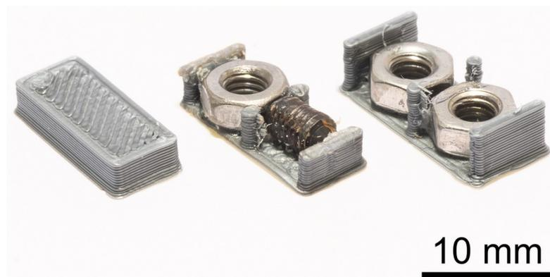
**Fig 1. Light, medium, and heavy (from left to right) dummy tags constructed based on the weights and dimensions of three commonly used radio transmitters.**
