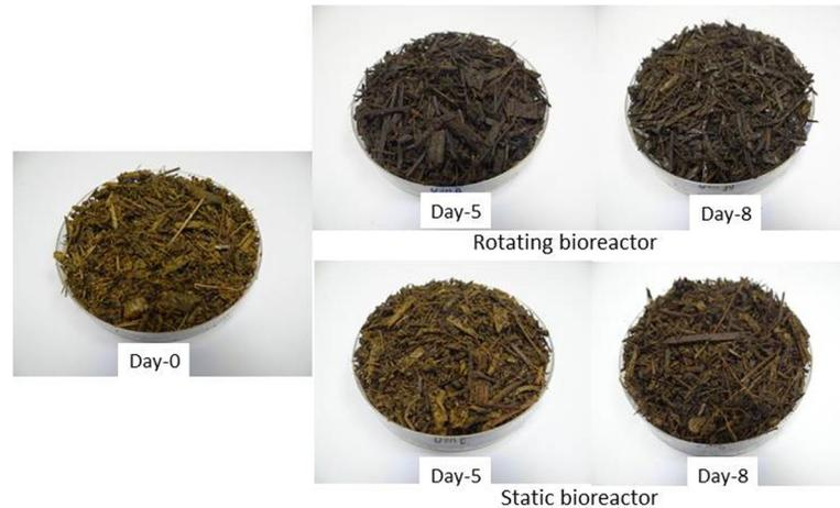
**Fig 7. Photos of compost material taken from the two bioreactors at days 0, 5 and 8 to show the changes in the color and material structure (visual testing).**
