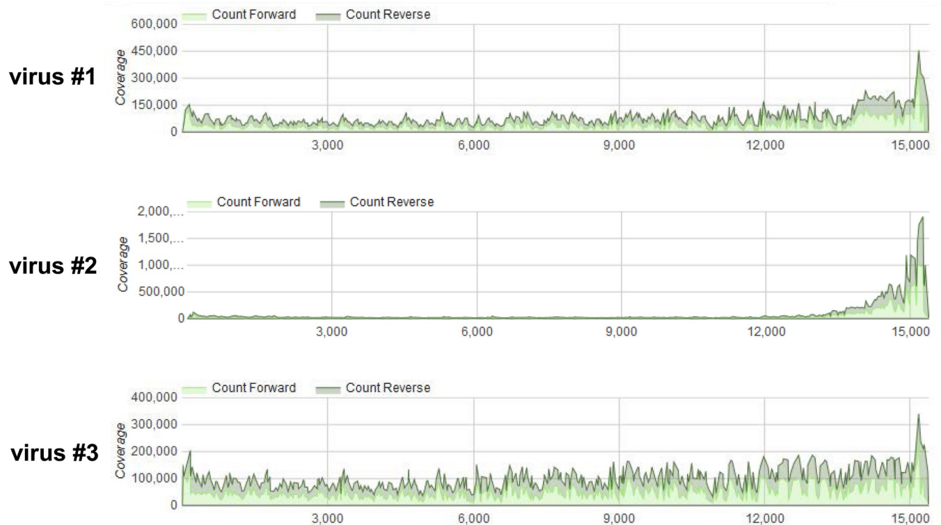
Fig 7. Differences in depth of coverage obtained by HTS from three recombinant MuV rescued from the same cDNA. Crude virus-containing cell culture supernatants were treated with Micrococcus nuclease followed by viral RNA extraction and high throughput sequencing using a HiSeq instrument. Data were analyzed using CBERs specialized high-performance integrated virtual environment (HIVE) platform. Note the steep increase in depth of coverage at the 5' end of virus #2 compared to viruses #1 and #3.
