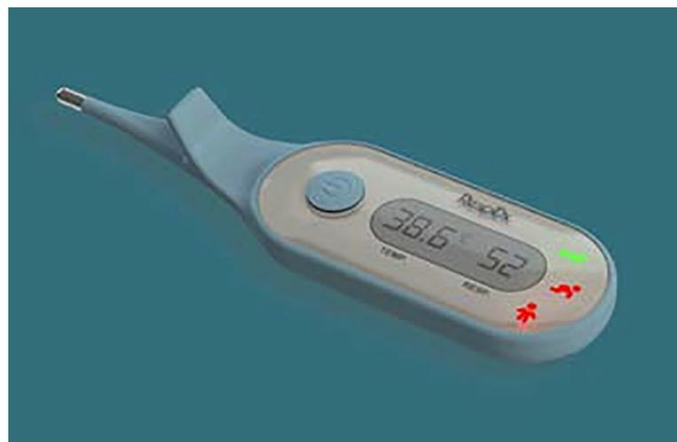
**Fig 1. First prototype of the Respirometer.**
