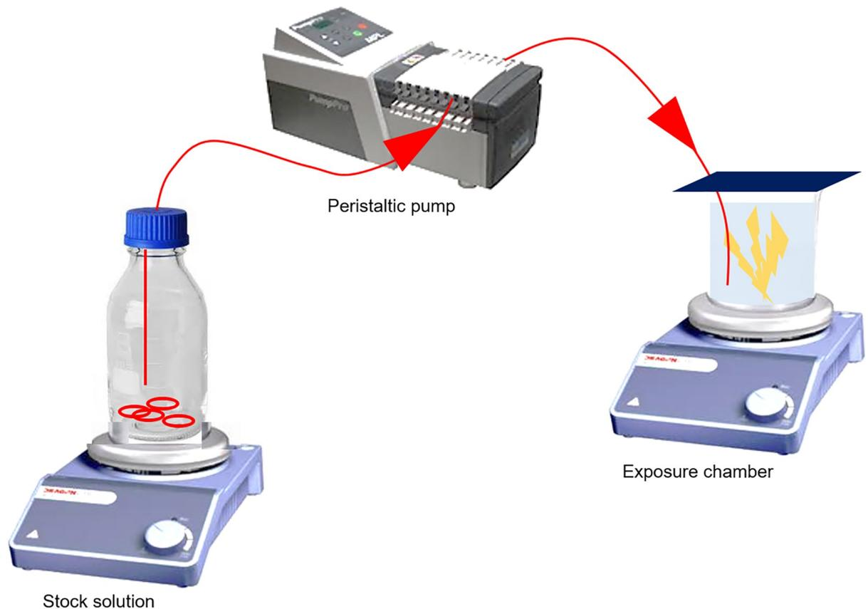
**Fig 1. Setup for 2-methylnaphthalene exposure.** Based on the principles of passive dosing described by Butler et al. [32], a passive dosage open system with flow-through using silicone O-rings has been developed. The peristaltic pump transfers stock solution from the stock bottle to the exposure chamber containing the test organisms.
