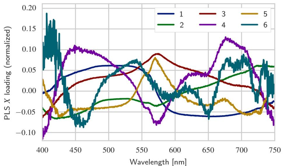
**Fig 7. PLS X loadings for orange corals.** Same as Fig 6, but created using data from orange corals. A notable difference is the significant noise in loading 6, indicating that explanatory power is decreasing at this point.
