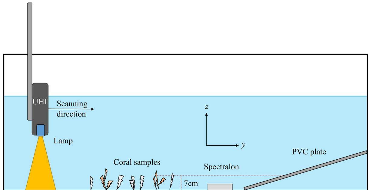
**Fig 3. Experimental setup for UHI image acquisition.** Samples of *L. pertusa* were set up on the bottom of a tank and imaged using an underwater hyperspectral imager (UHI). The UHI was attached to a linear scanning mechanism and operated in a “push-broom” fashion. The setup also includes a Spectralon reference plate and an inclined reference plate to account for changes in the spectrum due to the presence of water.
