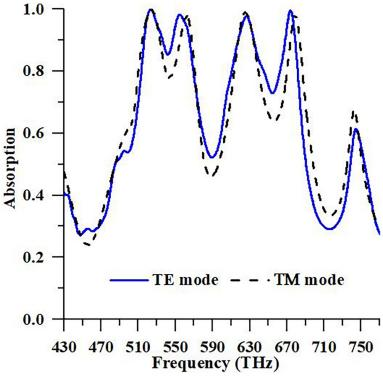
Fig 4. Numerical response of the proposed PMA in case of TE and TM polarization.
