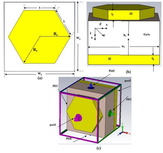
Fig 1. (a) Schematic diagram of PMA; (b) Unit cell with the bottom view; (c) Perspective view with boundaries.
