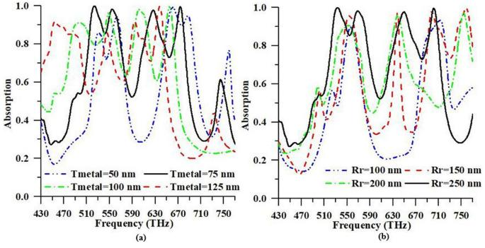
Fig 7. Absorption response of the proposed PMA for different (a) resonator and ground metal thickness (from 50 nm to 125 nm) and (b) radius of the resonator (from 100 nm to 250 nm).
