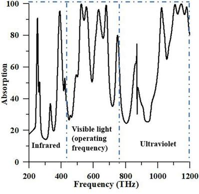
Fig 6. Absorption reply of the suggested PMA for whole sunlight.
