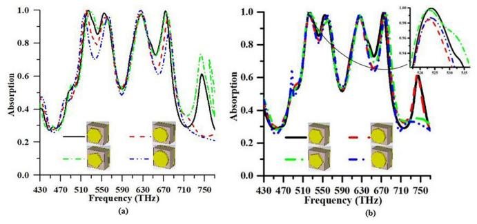
Fig 9. Absorption characteristic of the proposed PMA for different resonator shape such as hexagonal, octagonal, pentagonal, and circular with (a) the different effective area (b) the same effective area.
