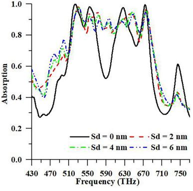
Fig 11. Absorption characteristic of the proposed PMA for different displacements like 0 nm, 2 nm, 4 nm, and 6nm between conducting materials.
