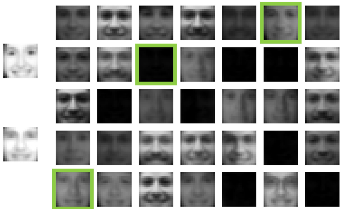
Fig 1. Face image reconstruction using features learned by NBMF. The five-by-seven matrix of images on the right shows the features that were learned. The two images on the left show the original image (top) and the reconstruction (bottom). The reconstruction is obtained by summing the features that are boxed in green. Note that although some of the features appear to be all black, they actually contain facial features that are small in magnitude (black corresponds to 0, white corresponds to 1).
