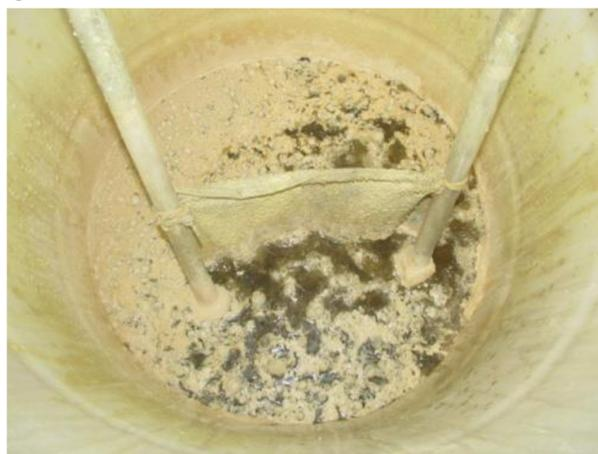
**Fig 4. Images of 104 L micro-aeration units.** A, View of insulated barrels. B, View of sulfur deposition on digestate surface in barrel receiving aeration. C, View of saturated fabric (29 x 29 cm) in barrels receiving aeration.
