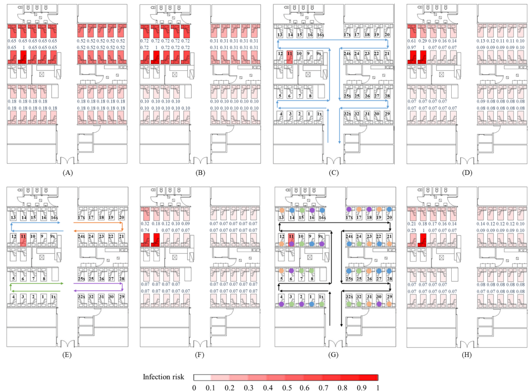
Fig 3. Distributions of reported attack rates and predicted infection risk and HCWs routine round patterns. (A) Reported attack rates distribution [20]. (B) Predicted average infection risk distribution (for 1,000 simulations) via the long-range airborne route at 24:00 on March 12, the end of the exposure period. (C) HCWs routine round Pattern 1. (D) Predicted average infection risk distribution via the fomite route (Pattern 1). (E) HCWs routine round Pattern 3. (F) Predicted average infection risk distribution via the fomite route (Pattern 3). (G) HCWs routine round Pattern 5. (H) Predicted average infection risk distribution via the fomite route (Pattern 5). The largest virus-containing droplet size d_g = 100 \mu\text{m} , dose-response parameters in respiratory tracts \eta_r = 3.2/\text{mRNA copy} and on mucous membranes \eta_m = 3.2 \times 10^{-3}/\text{mRNA copy} and the viral load coefficient c_L = 10 . Bed numbers are marked in black in (C), (E) and (G). Reported attack rates and predicted average infection risks for every inpatient are marked in blue in (A), (B), (D), (F) and (H). The intensity of red shading represents levels of attack rate or infection risk.
