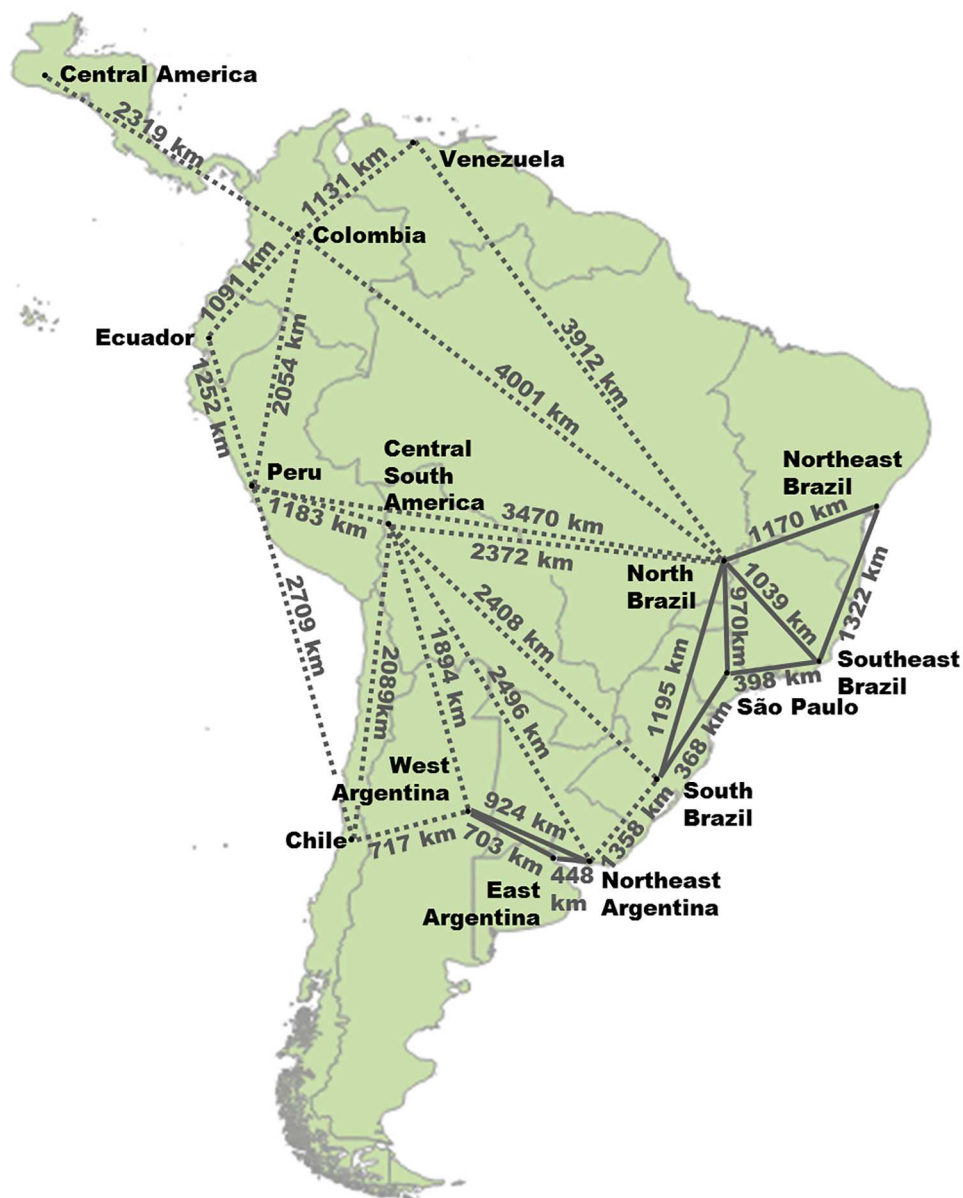
Fig 3. South and Central American sub-regions and HVDC transmission lines configuration.
