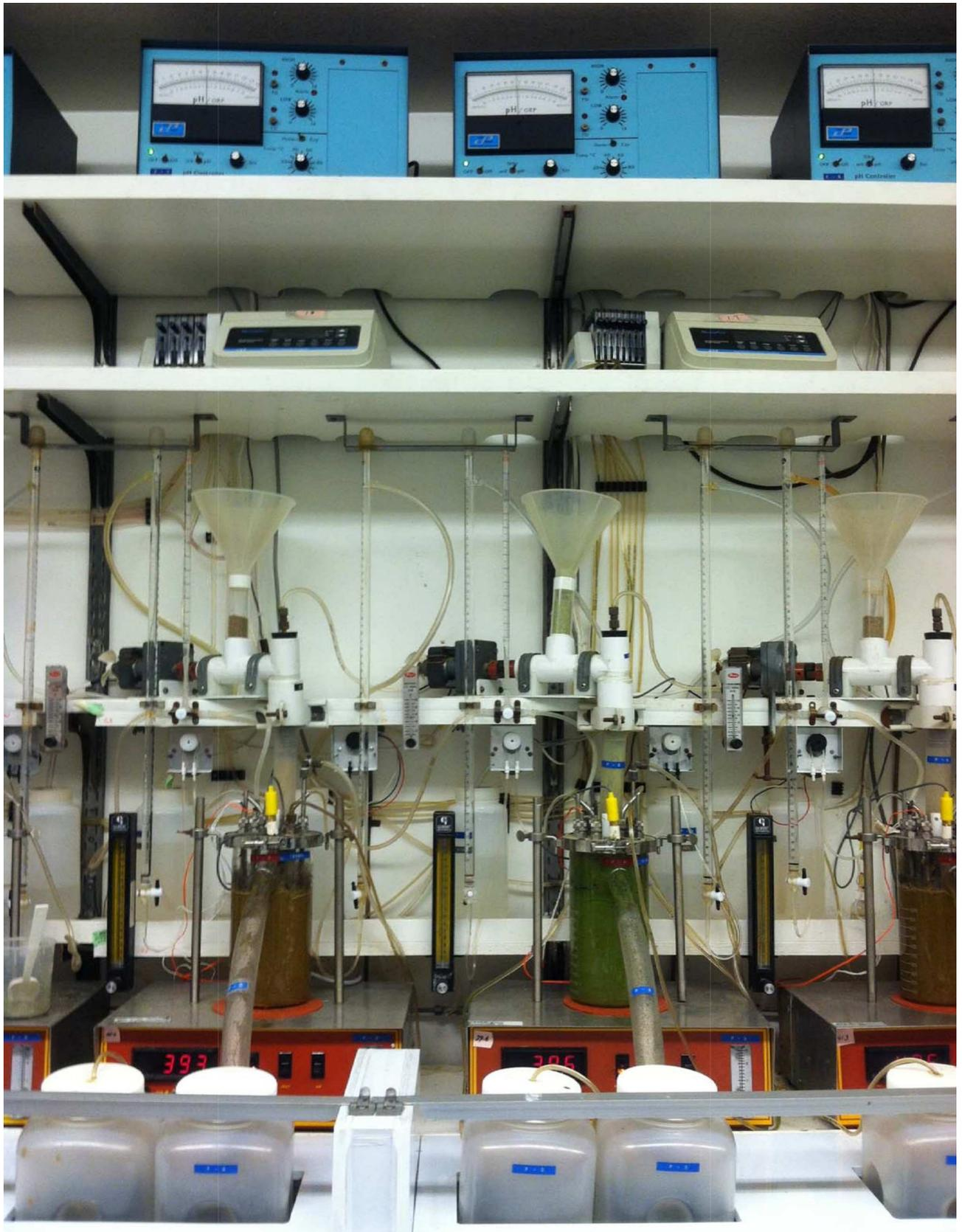
**Fig 3. Dual-flow continuous culture system frontal view.**
