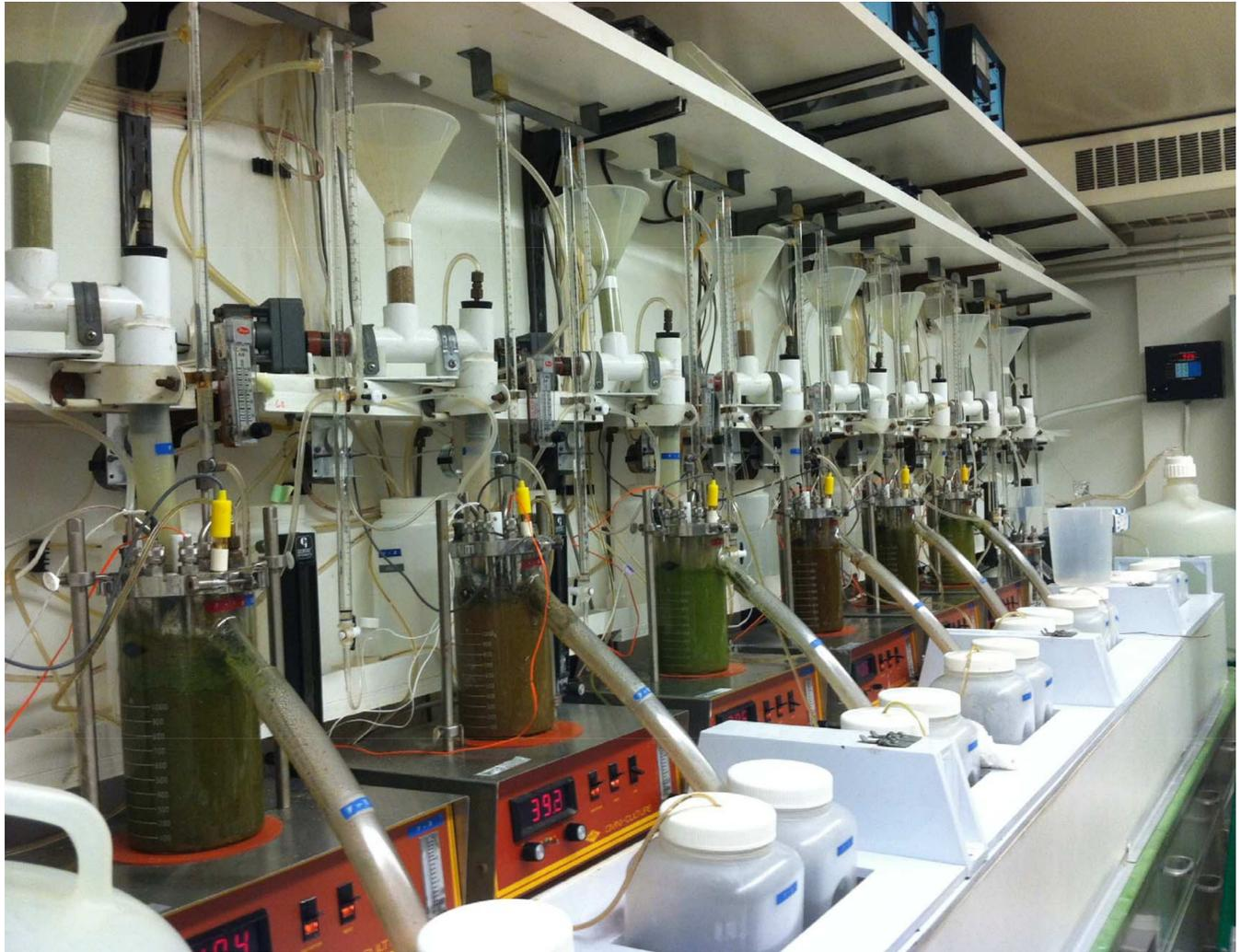
**Fig 1. Dual-flow continuous culture system right view.**
