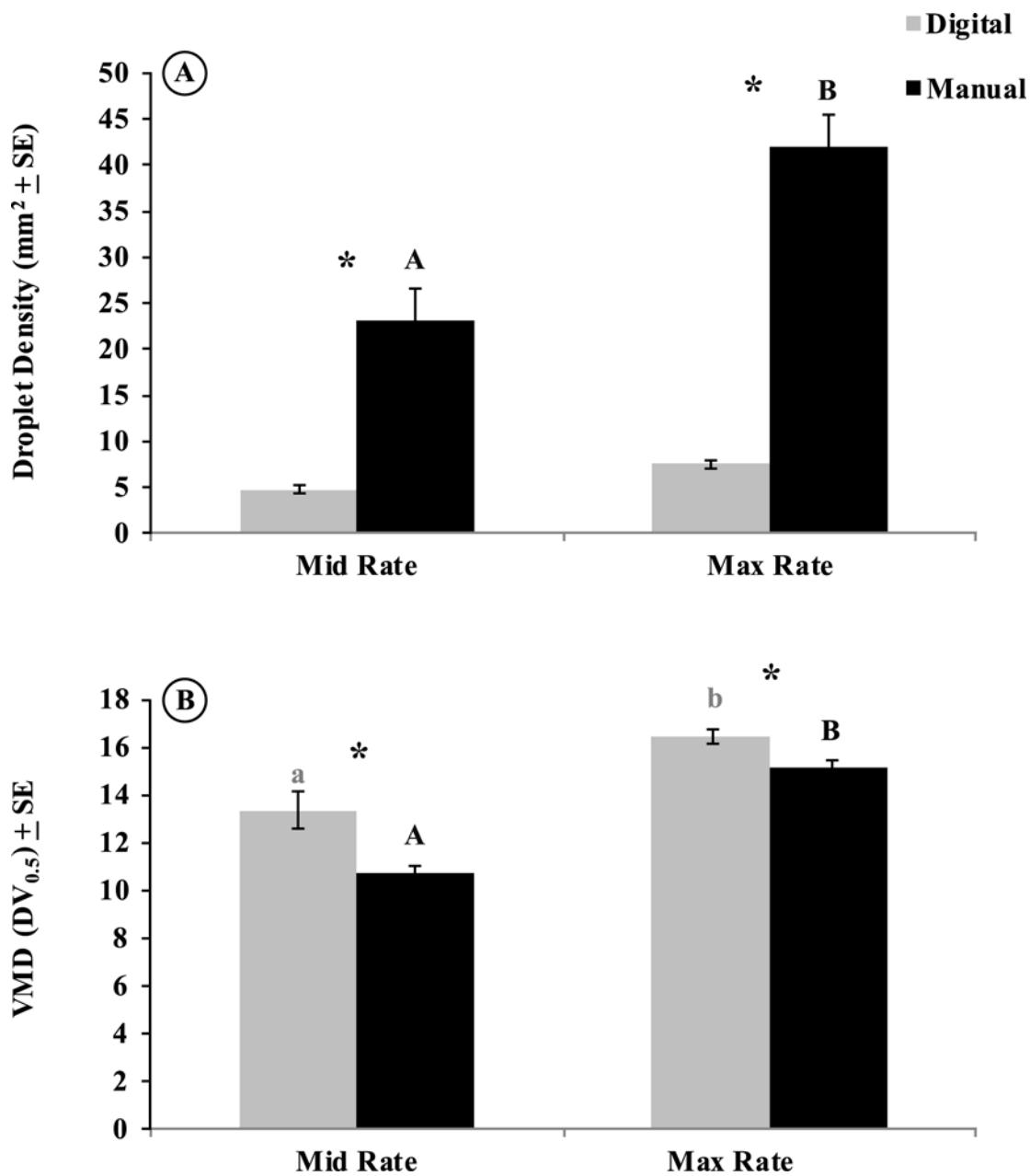
**Fig 5. Combined droplet density (drops per  $\text{mm}^2$ ) and volume median diameter ( $\mu\text{m}$ ; VMD) of spray plume from all sampling stations in urban Mercer at two different application rates sampled by Hock impactors and recorded by two analysis methods (digital and manual). Treatments with different letters and asterisks denote significant differences by ANOVA ( $P < 0.05$ ).**
