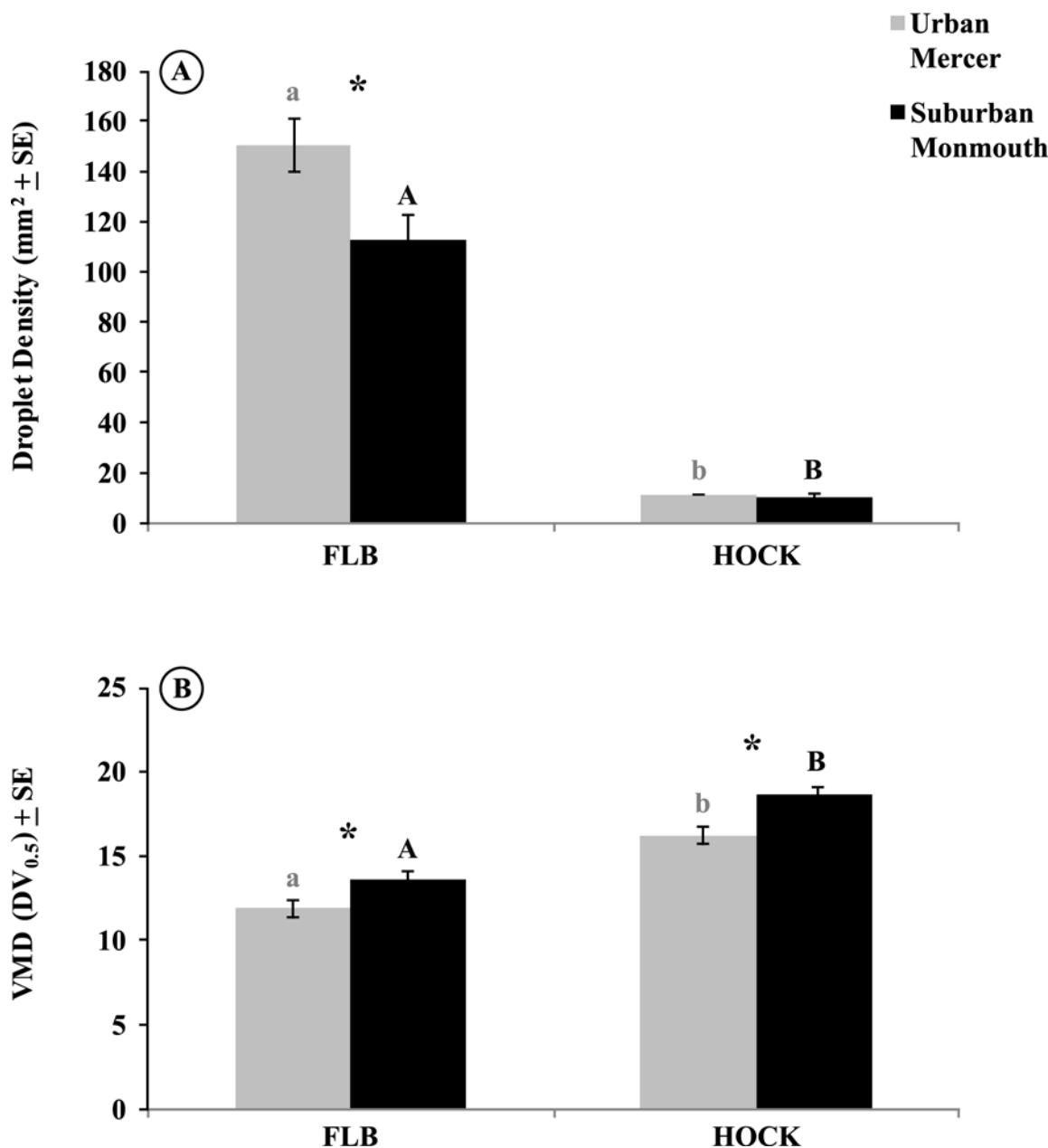
**Fig 4. Combined mean values for droplet density (drops per  $\text{mm}^2$ ) and volume median diameter ( $\mu\text{m}$ ; VMD) of spray plume from all sampling stations in urban Mercer and suburban Monmouth sampled by both impactor types (FLB and Hock). Treatments with different letters denote significant differences within county by impactor type and asterisks denote significant differences between counties by ANOVA ( $P < 0.05$ ).**
