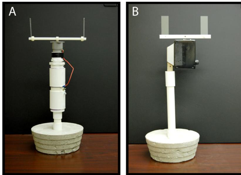
**Fig 3. Rotating impactors used for droplet sampling of adulticidal spray plumes.** A) Florida Latham Bonds (FLB) rotary-type impactor with 3 mm rods. B) Hock rotary impactor with 25 mm microscope slides.
