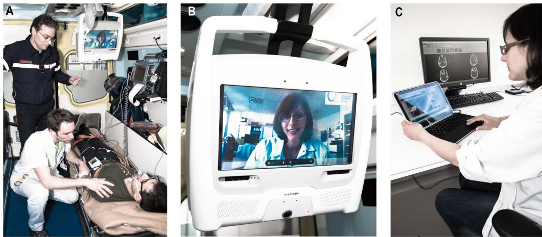
Figure 1. The PreSSUB 3.0 system. The telemedicine device is securely mounted to the ceiling of the ambulance (A) and allows bidirectional audiovisual communication between the patient and the teleconsultant via integration of a microphone, speakers, a screen and a 360° view camera (B). The teleconsultant has mobile access to the telemedicine platform using a lightweight laptop computer with touch screen, integrated microphone, speakers and a webcam (C). doi:10.1371/journal.pone.0110043.g001
