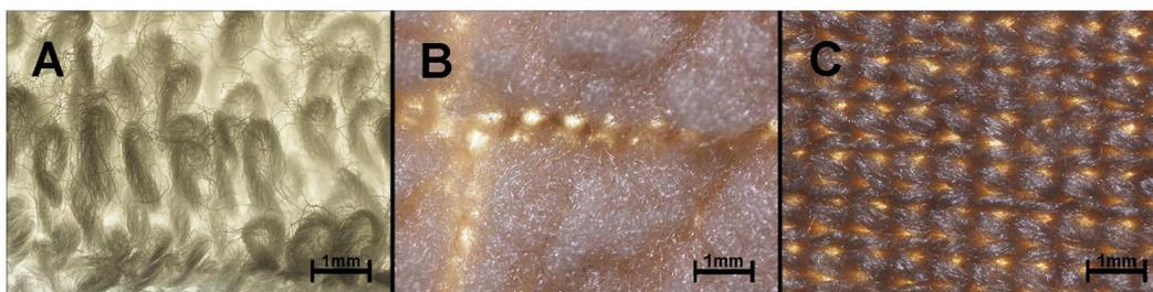
**Figure 1. Micrographs of fabrics used for THS extraction.** (A) Terry cloth is a loosely knit fabric made of loops of cotton which increase its surface area tremendously and contribute to the absorption of THS. (B) Polyester is a more tightly knit fabric with one fuzzy surface and (C) one compact tightly woven surface.
