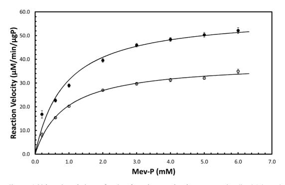
**Figure 4. Initial reaction velocity as a function of mevalonate-5-phosphate concentration.** Closed circles are data for incubation at 37°C and open circles are data for incubation at 30°C. doi:10.1371/journal.pone.0087112.g004
