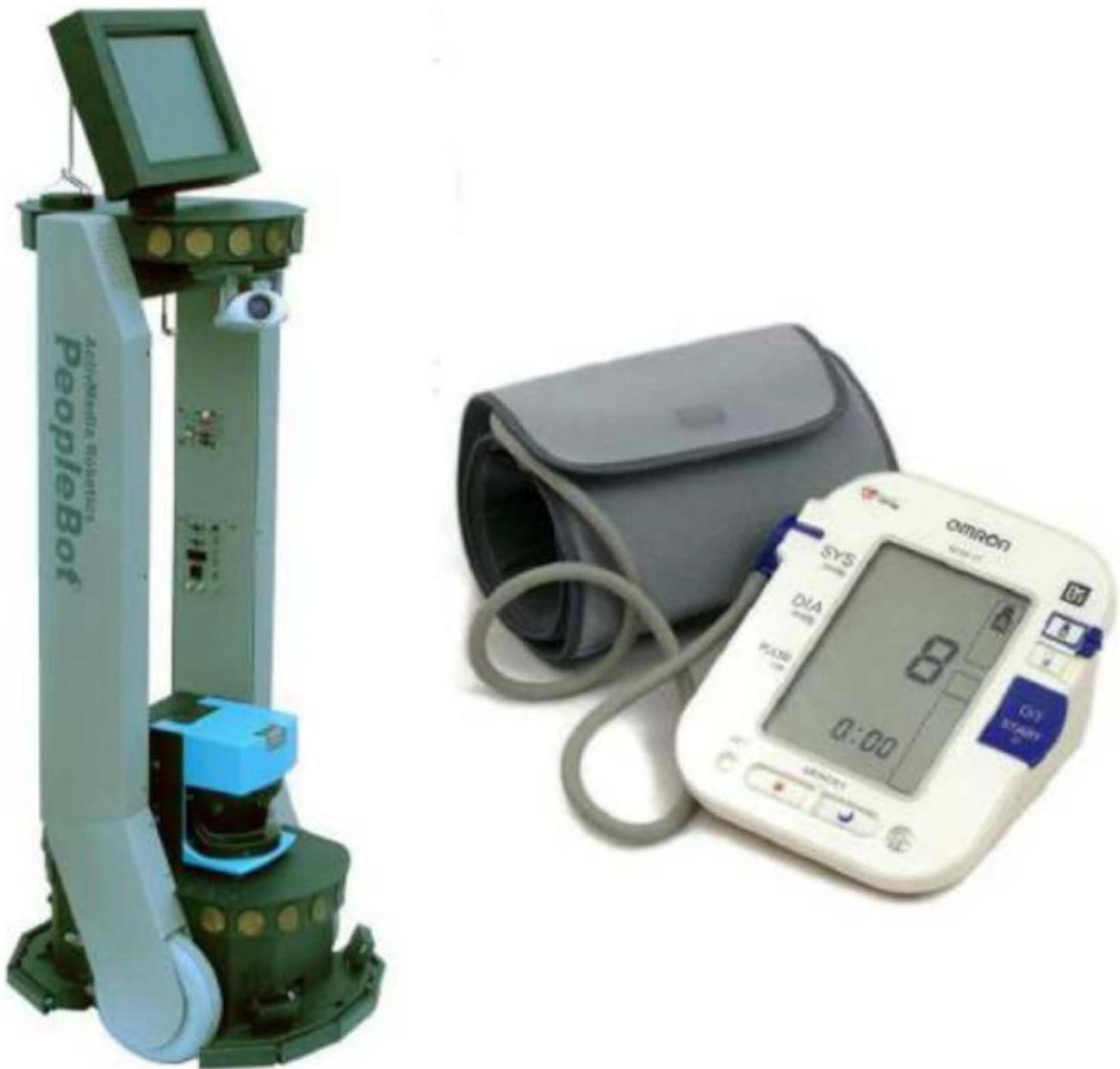
**Figure 1. Peoplebot robot and blood pressure monitor that was attached to it for the study.**
