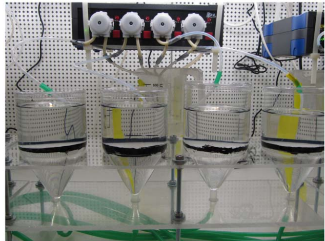
Figure 2. The experimental set-up. The flow-through testing apparatus, showing four experimental units (volume, 500 mL) with five D. magna each. Approximately 40 mL of the test medium was introduced every other hour slightly below the surface of the water. The old test medium was passively discharged using hydrostatic pressure at the bottom of each vessel. A fine mesh screen (0.1 mm) prevented the loss of recently hatched juvenile daphnids.
