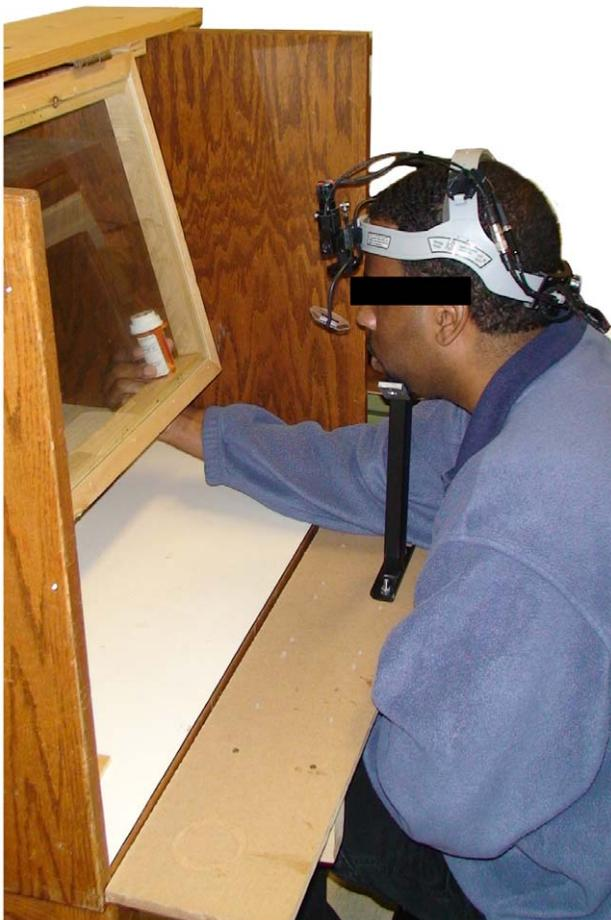
**Figure 5. Experimental set up (chin rest, calibrated plane and the head-mounted optics of our ASL 501 eye tracking unit).**
