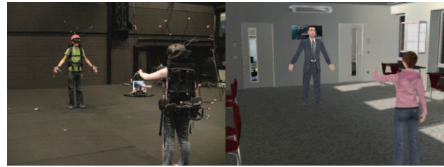
Figure 7. The experimental setup. Left: The participants wore a total of six tracked objects ( 2 \times hands, 2 \times feet, backpack and helmet). Right: the corresponding virtual environment, showing the avatars in the self-animated third-person perspective. doi:10.1371/journal.pone.0025759.g007
