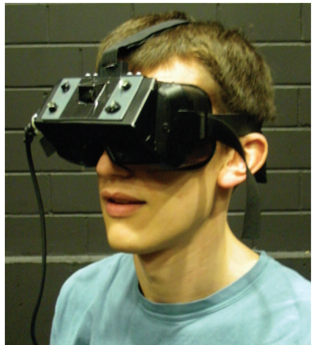
Figure 8. Head-mounted display. Participants wore an eMagin HMD mounted in goggles, so they could see the virtual world and not the real world. doi:10.1371/journal.pone.0025759.g008
