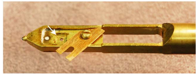
Figure 4. Picture of the tip of the modified specimen holder (Hitachi type). The liquid enclosure fits into the slot indicated by the arrow. A metal blade and a screw serve to fix the liquid enclosure in place.
