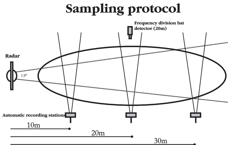
**Figure 1. Sampling protocol of experimental trials carried out at 20 independent sites from July to September 2007.** At each site bat activity was recorded for 1 h at three distances from the radar antenna (10,20,30 m) using three automatic bat recording stations orientated perpendicular to the radar beam. A frequency division bat detector was positioned 20 m from the radar antenna to provide further information on bat foraging activity during this period.
