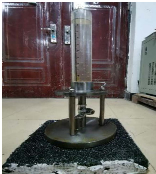
Fig 9. Pavement permeability test.
