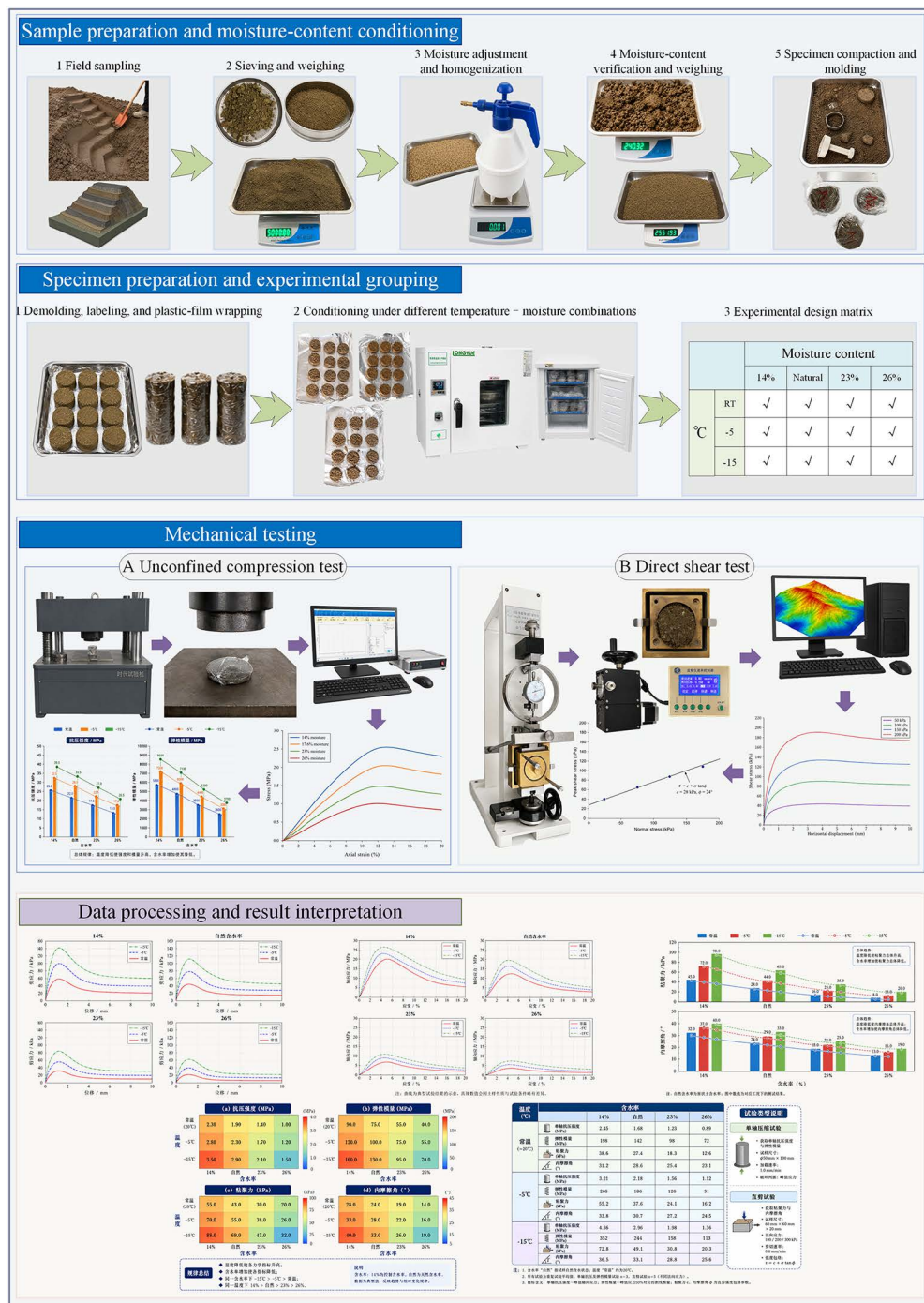
Fig 4. Workflow of specimen preparation, mechanical testing, and data analysis under different temperature–moisture conditions. All photographs, plots, screenshots, and diagrams in this figure were created by the authors.
