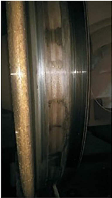
Fig 1. Picture of wheel polygonal wear.
