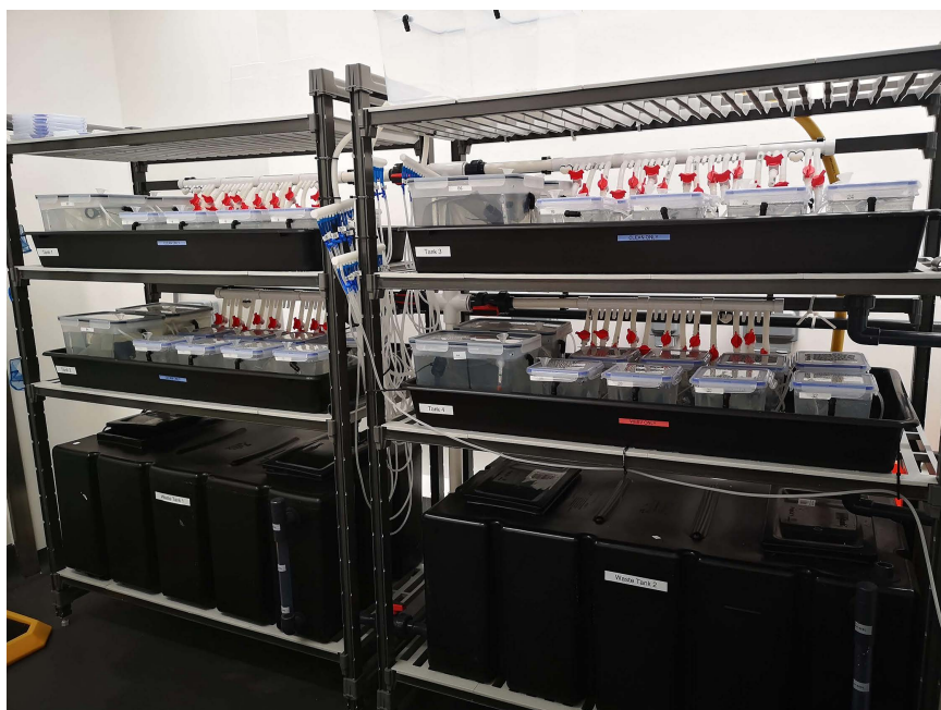
Fig 1. Shrimp holding facility. The picture shows the RAS system setup used for the viral challenges in adult L. vannamei shrimp. Each tank is fitted with an individual aeration system. A small-scale RAS system is used to keep the water parameters constant and water quality within safety levels. The feeding was done manually.
