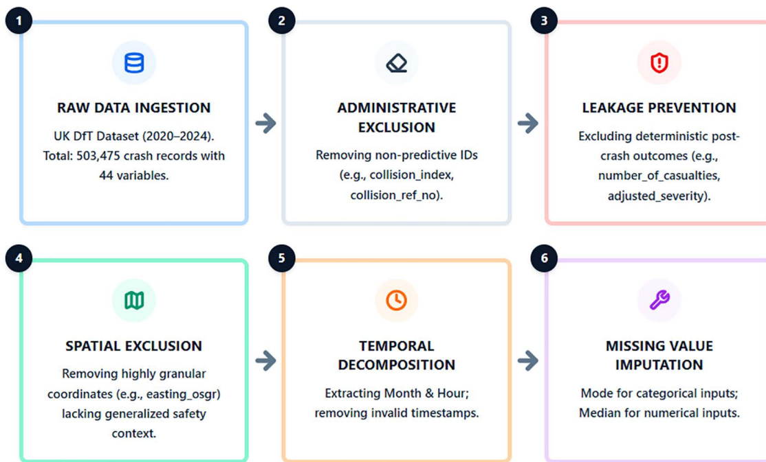
Fig 2. Data cleaning pipeline and feature extraction strategy.
