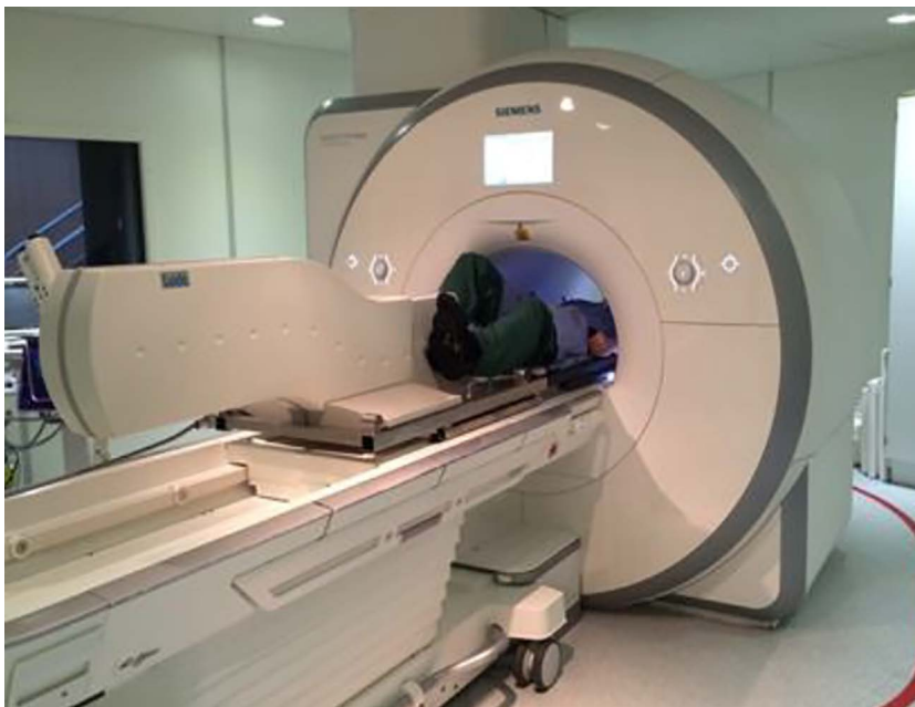
Fig 1. Experimental setup for cycle ergometer (Lode BV, Groningen, The Netherlands) used for exercise CMR.
