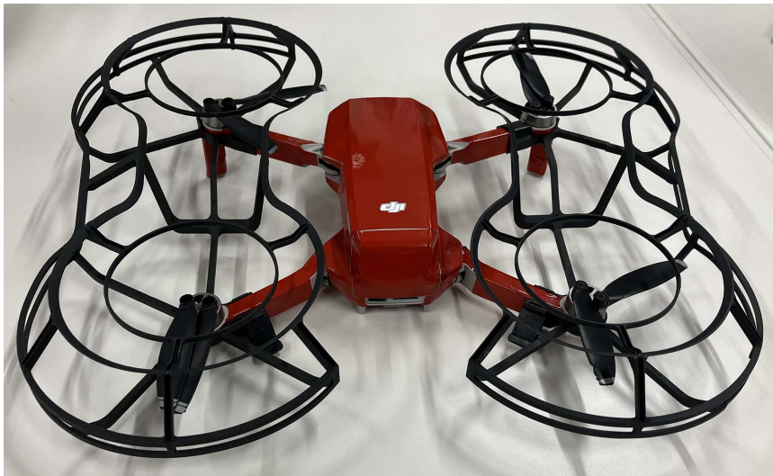
Fig 6. Modified commercial drone (DJI Mini2) for improved detection. Red stickers are applied to the surface of the compact and lightweight DJI Mini2.
