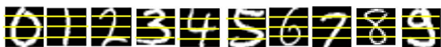
Fig 3. Image partitioning into four horizontal segments. Each digit image is divided into four horizontal parts to extract localized ECDF features.
