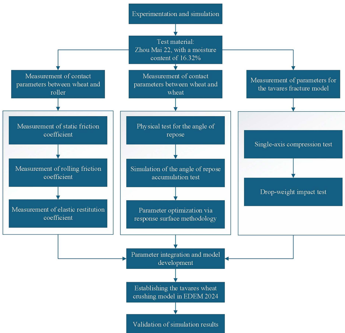
Fig 2. The schematic workflow of experimental and simulation steps.
