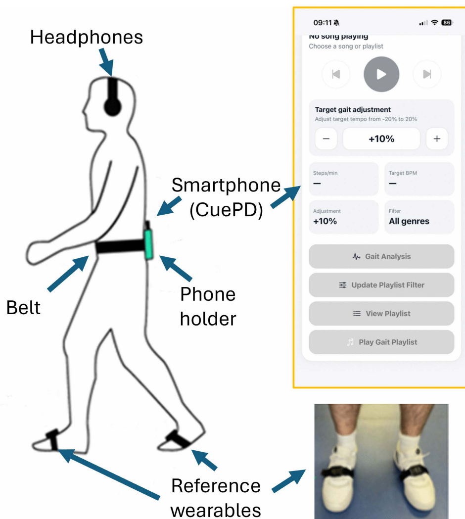
Fig 1. Equipment Configuration for the Study. This figure displays the setup of the smartphone device with CuePD installed, reference IMU wearables, a pair of wireless headphones, a belt, and a phone holder as used in the experiments.
