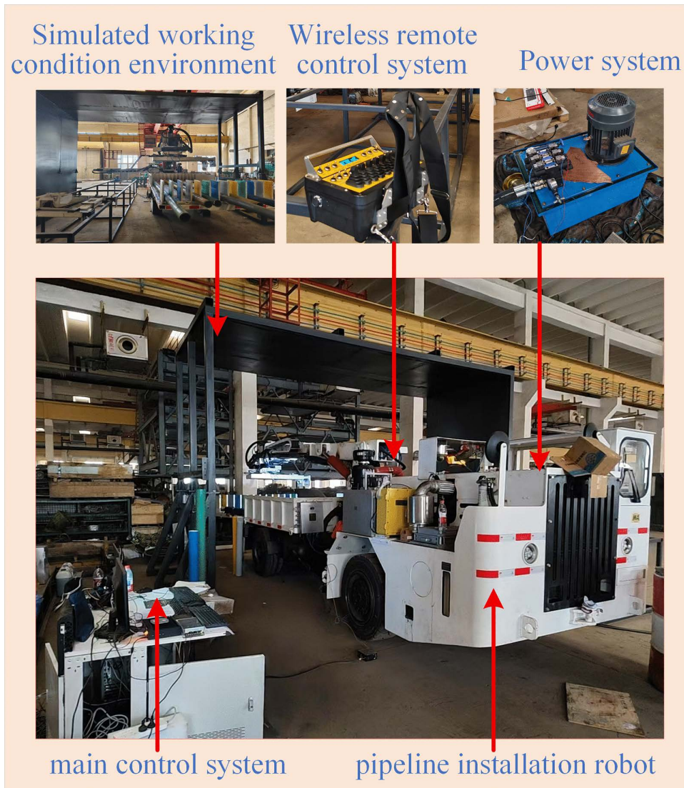
Fig 18. Experimental platform of pipeline installation robot.
