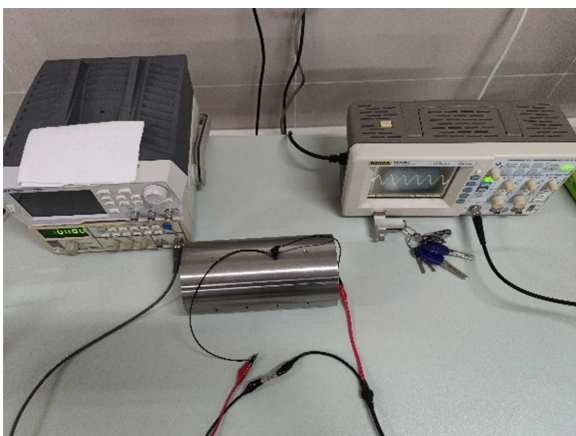
Fig 11. Eddy current testing experimental platform.
