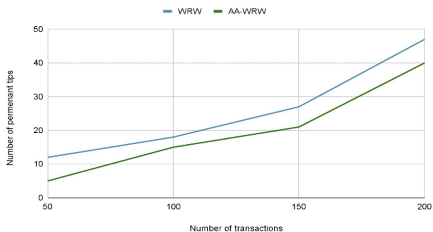
Fig 13. Evolution of the Number of PT in the addTransportation Function. The figure compares the number of permanent tips (PT) versus the total number of transactions for two tip selection algorithms: WRW and AA-WRW in the addTransportation function.
