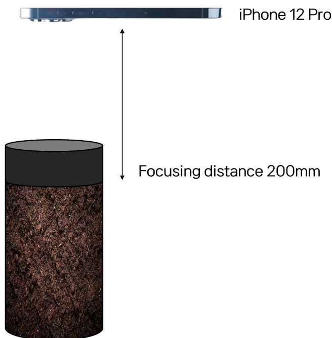
Fig 4. Camera Setting for in situ image acquisition.
