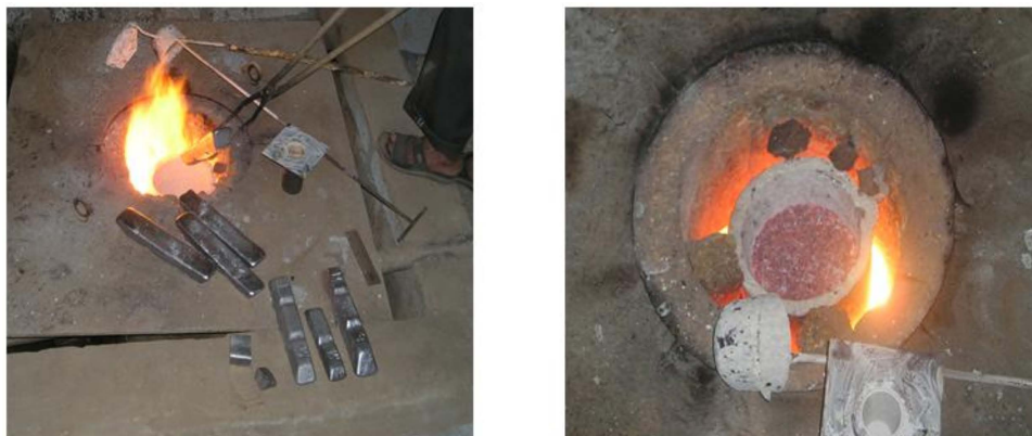
Fig 5. Oil-fired diesel furnace of the pit type for alloy melting.
