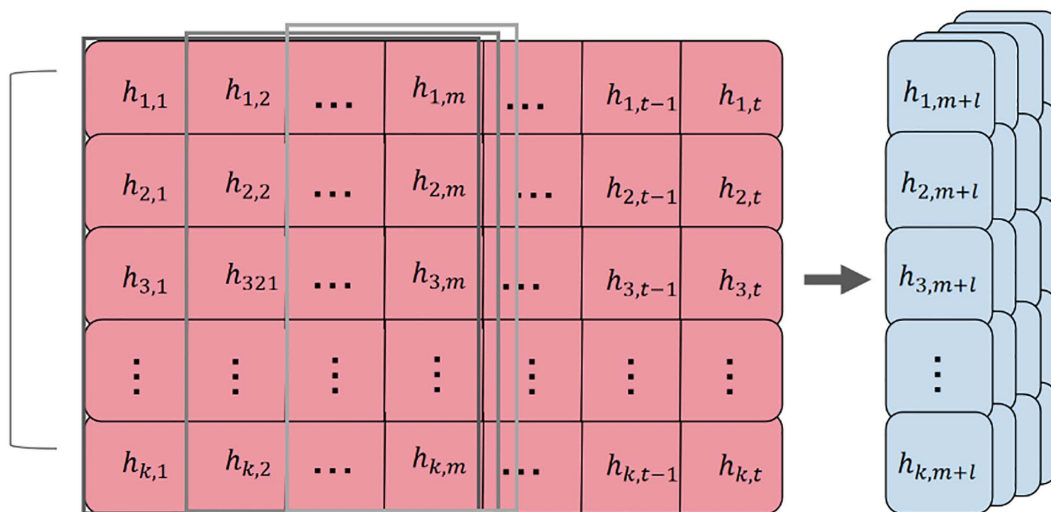
Fig 1. Schematic diagram of sample slicing for multidimensional historical health index sequence data.
