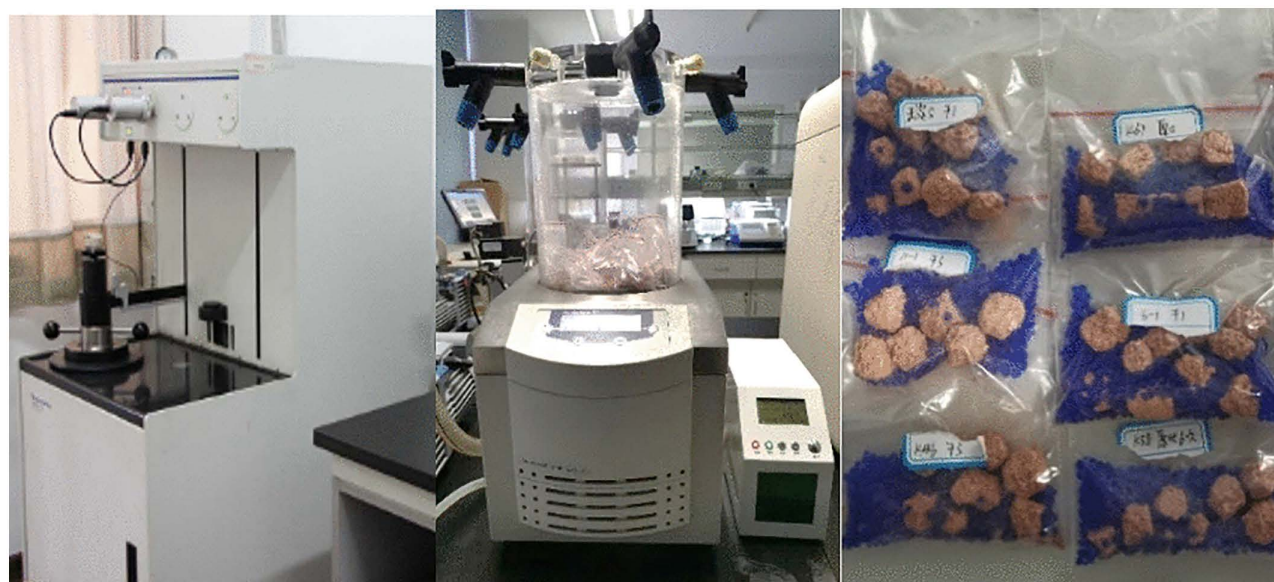
Fig 3. Equipment and specimens in MIP test. (a) Mercury porosimeter (b) Vacuum freeze drier (c) Freeze-dried specimens.
