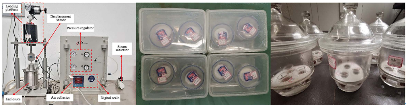
Fig 4. Equipment used in SWCC test. (a) GEO-Experts pressure plate system (b) Insulated box in FPM (c) Equipment used in VEM.
