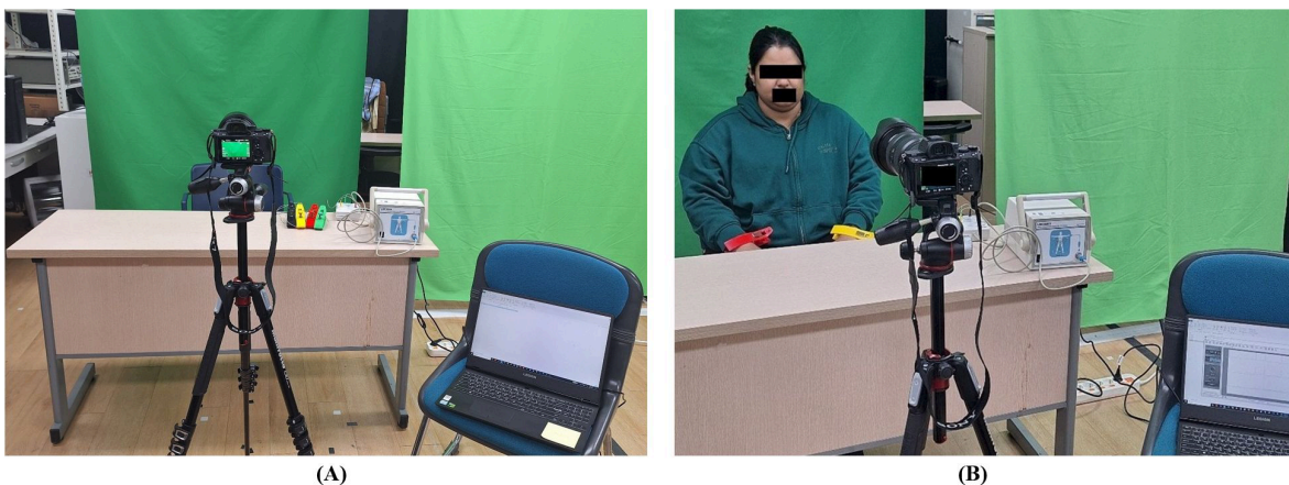
Fig 2. Experimental setup and dataset collection. (A) Overview of the experimental setup, (B) Custom database collection while the subject sitting from 1 m away from camera and corresponding reference HR measurement are performed using QECG sensor.
