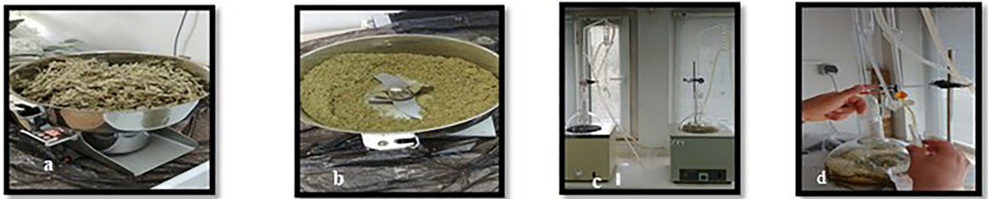
Fig 2. a. b Powdering of O. majorana , c. Clevenger Device (double), d. Essential oil from O. majorana .
