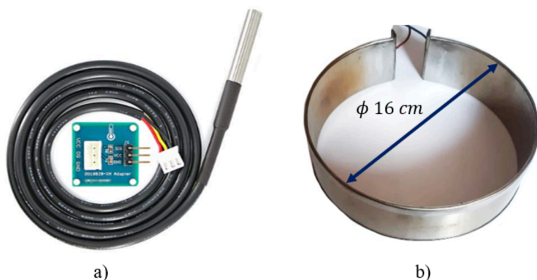
Fig 6. Temperature system components. A) DS18B20 temperature sensor. B) Armored resistor.
