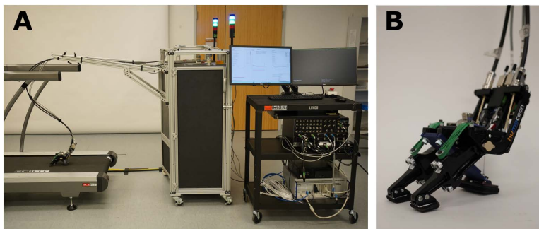
Fig 3. Prosthetic foot emulator. (A) Two off-board actuators control the sagittal and coronal stiffness properties of the (B) prosthetic end effector by manipulating the torque produced by the two toes of the end effector.
