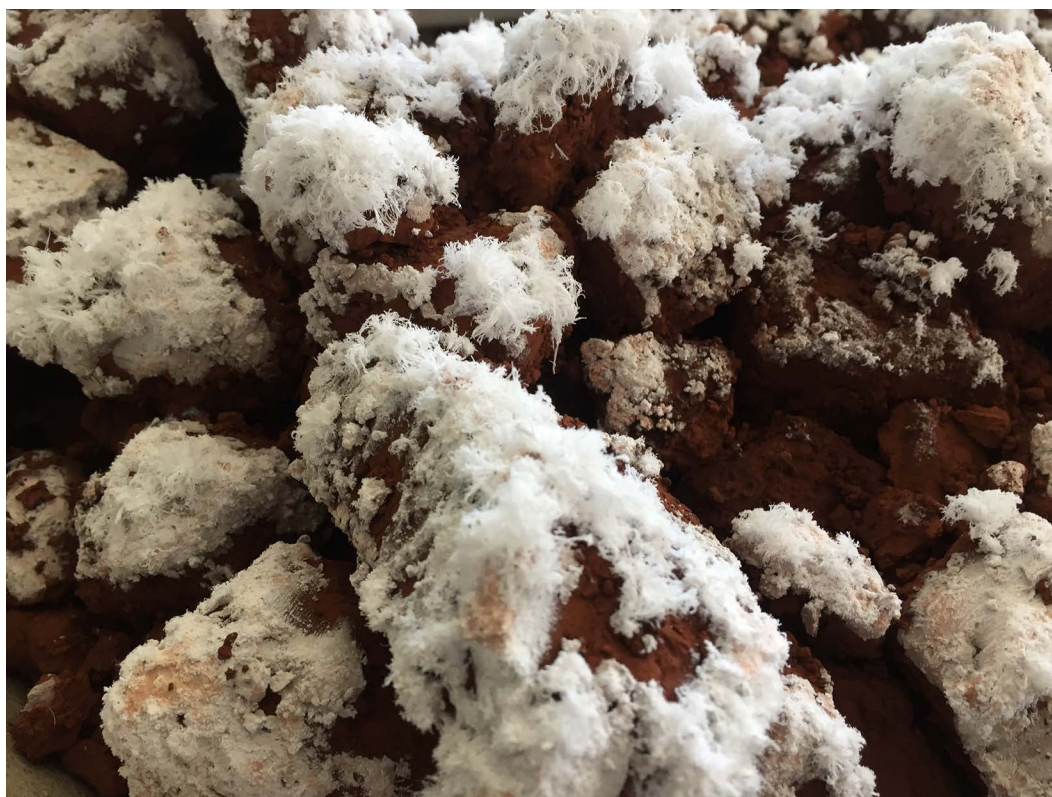
Fig 3. White crystal formations observed on the surface of air-dried RM samples.
